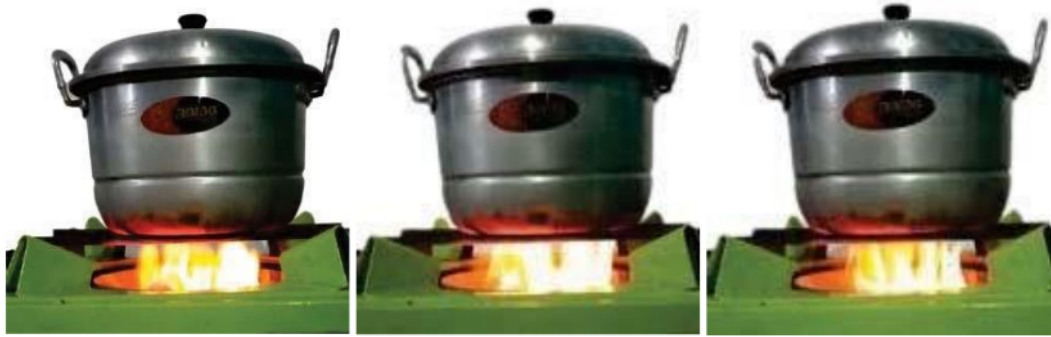
FIGURE 6. Flame stability of the briquette stove using an adjuster.
