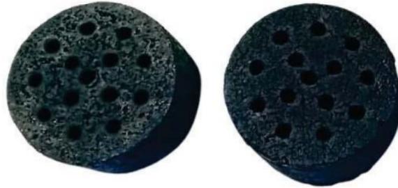
FIGURE 2. Sago waste briquette
