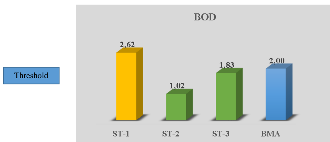
Figure 4. Parameter Diagram of Biological Oxygen Demand (BOD) Index Sentani Lake Water and Water Quality Standards
