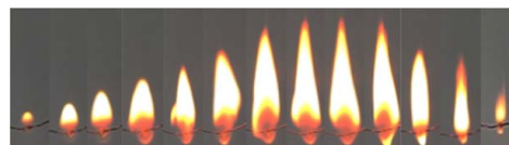
Fig. 7. Flame evolution of CCO with 300 ppm EO
