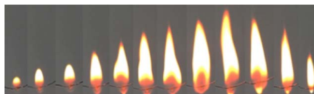
Fig. 6. Flame evolution of CCO with 100 ppm EO
