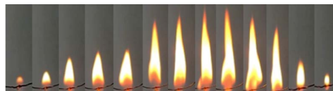
Fig. 11. Flame evolution of CCO with 300 ppm CvO
