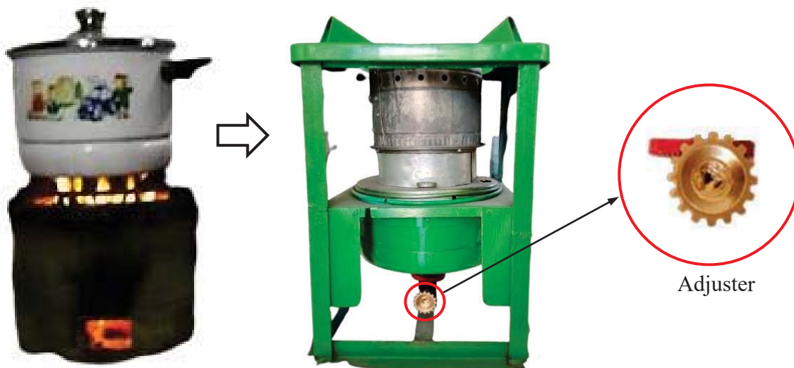
FIGURE 3. Development of a briquette stove model with an adjuster.
