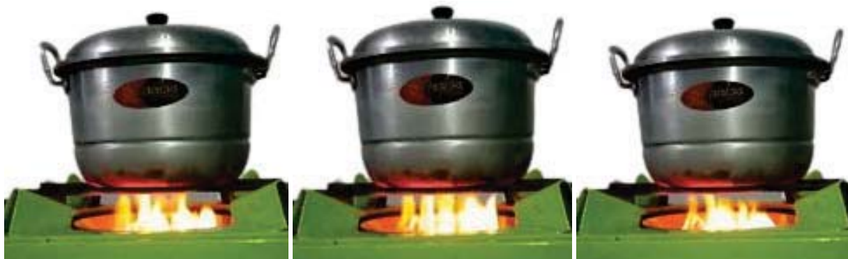
FIGURE 5. Flame stability of the briquette stove without used an adjuster.
