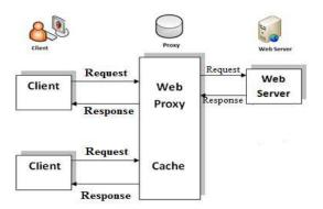
Fig. 2. Performance Mechanism Cahe Proxy
